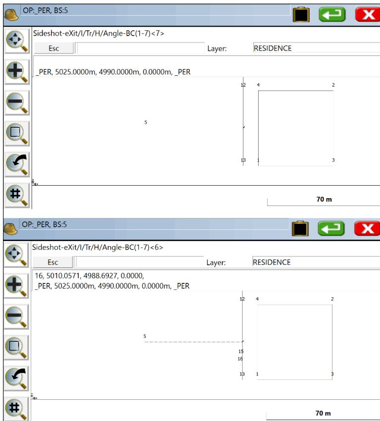
Note that at the Angle/Bearing prompt, you can transition back to inverse (from your occupied point) or to traverse, which would move you up to the next traversed point. Code 7 turns angle right. In the standard MAP screen prior to selecting T or SS, if you click the lower left View Options button, and then select the Data tab and choose Traverse Defaults, you can turn on the Zenith Angle or Elevation Difference prompts.
