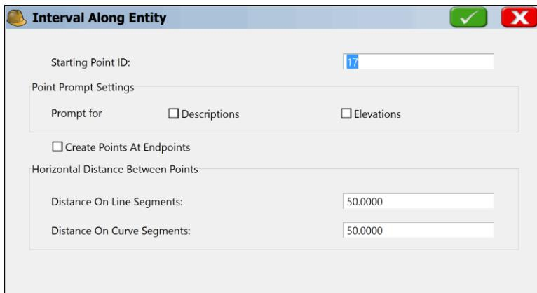
This command is often used for creating points on centerlines. Note the program resets the interval at break points like PI's and PC's. Note that you can choose to create more points at a smaller interval going around curves.
