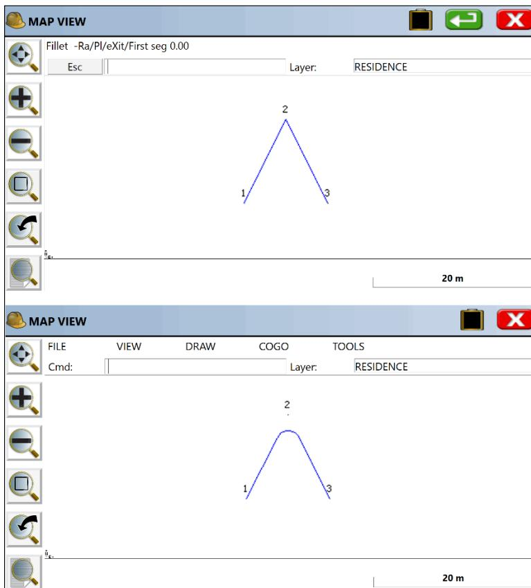
See the above two figures. Because in the Left figure, from 1 to 2 to 3 was one continuous polyline, after the radius was set at 15, P was entered to set up the one-pick approach for polylines, leading to the completed fillet command and the result as shown in the Right figure. Now you can do Cogo, Interpolate Points, Polylines to Points (P2P) and solve for the points for the beginning of the arc, radius and end of arc, for purposes of stakeout (set out).
