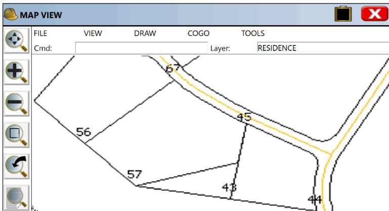
Note how the hinged side occurred on the clockwise side of the polygon perimeter (side 57 to 43). If we erase the new polyline, reverse the original polyline (RV) and repeat the command, this time answering “No” to “Keep existing” and again targeting 24000 Sq. Ft. area, we get the following:
