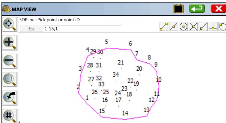
Finally, if you are doing a stockpile and make the effort to put this outer perimeter in the “Perimeter” layer, then you can select the “Stockpile” option within Volume, define the final surface appropriately, and click OK. You don't need any other definition for the original surface. This is because the Perimeter layer will define both the inclusion perimeter and the original surface in this case.
