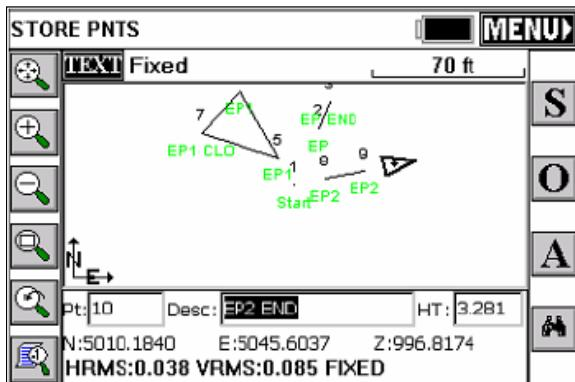
The above figure displays the next EP code EP2 stored using GNSS Simulation. When ended with a END or CLO description after EP2 SurvPC will prompt for EP GIS data to attach to the polyline as defined above.
