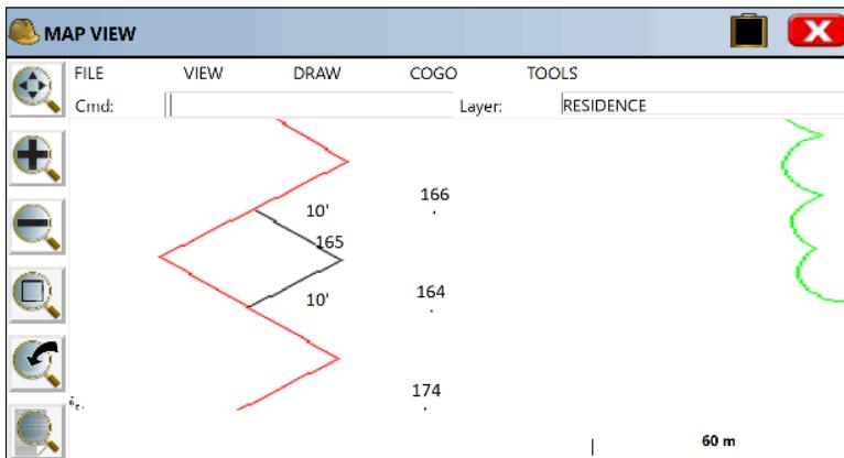
For L-shaped figures, offsets are also projected through to the other side, so that the offset for point 174 appears across the building, for purposes of pulling a stringline.
