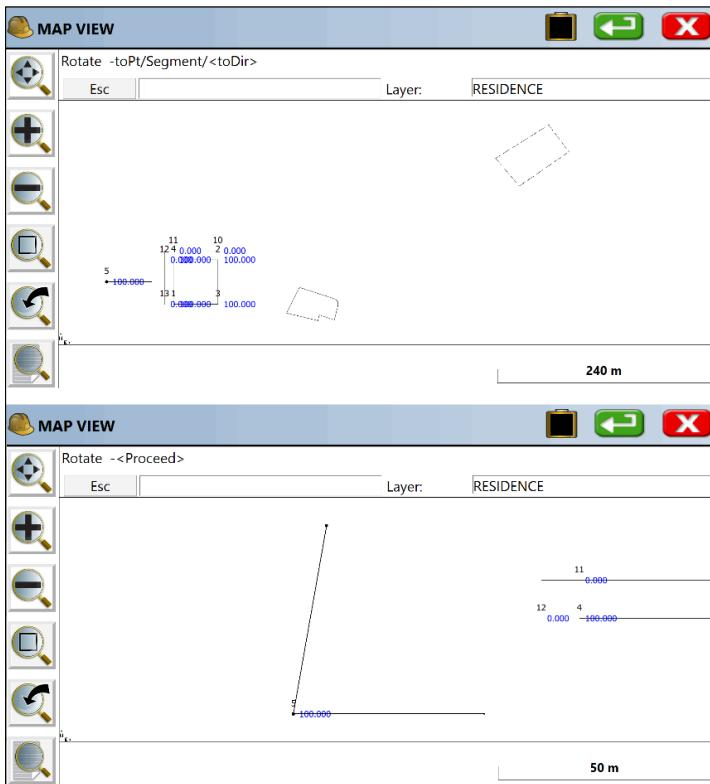
After the rotation is confirmed, you obtain the final results shown below. The simplest rotation, of course, is just by angle, where 10 degrees would rotate 10 degrees clockwise from the pivot point.
