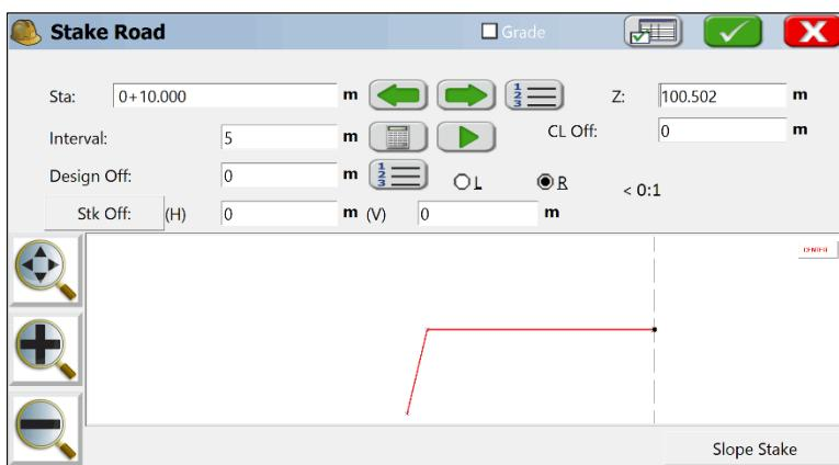
Using the "Interval" method (normal method), vertical offsets can be by elevation difference (default), or by slope percent or ratio. The default "Continuous" option keeps the offset 3D Polyline as a single entity. If you do the "Segment" option approach, only the segments of the 3D polyline will offset (leaving gaps), and you have the option to create Point IDs on the offset vertices.
