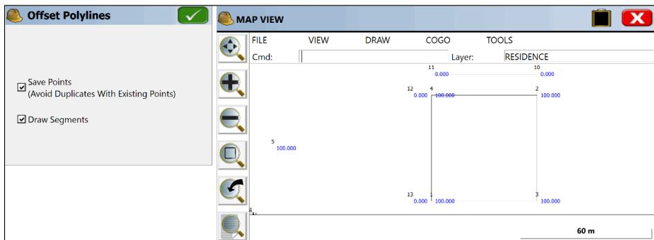
For L-shaped buildings or figures with angles, an additional interior offset point is calculated at the intersect of the parallel offset lines based on the entered offset distance, such as 10 (see point 165 below--the lines to 165 are drawn only to illustrate the 10' offset):
