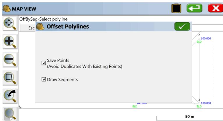
The "Constant" option takes a 3D polyline and offsets it to a constant elevation for all vertices. So if you measured the base of a retaining wall that sloped downhill, but the top of the wall was a constant elevation, you could offset a fixed horizontal distance to that single elevation.
