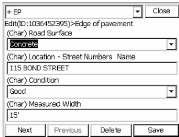
The figure above displays the ease of reviewing, creating or editing GIS data using Input-Edit GIS Data. From the MAP screen Input-Edit GIS Data was selected and the closed 3D Polyline picked on the screen. The GIS data stored prior was displayed for review or editing. Any data point, polyline or closed polyline could be selected using the Input-Edit GIS Data command in MAP and new GIS attached to this entity or existing GIS data reviewed and edited.
