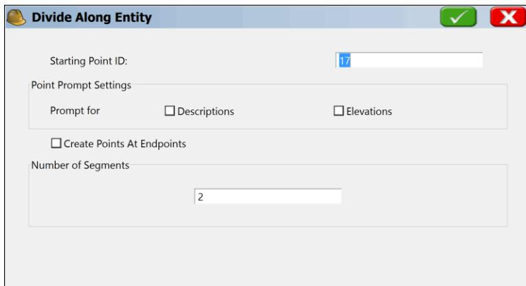
The command will create new vertices along the polyline but can also create point numbers starting at the entered Point ID, and you can elect to be prompted for descriptions and/or elevations at each new point. If a property line were divided into two segments, you would create three new points, if Create Points at Endpoints is clicked on. Otherwise, division of a line into two segments would create only 1 new point ID, in the middle of the line or polyline.
