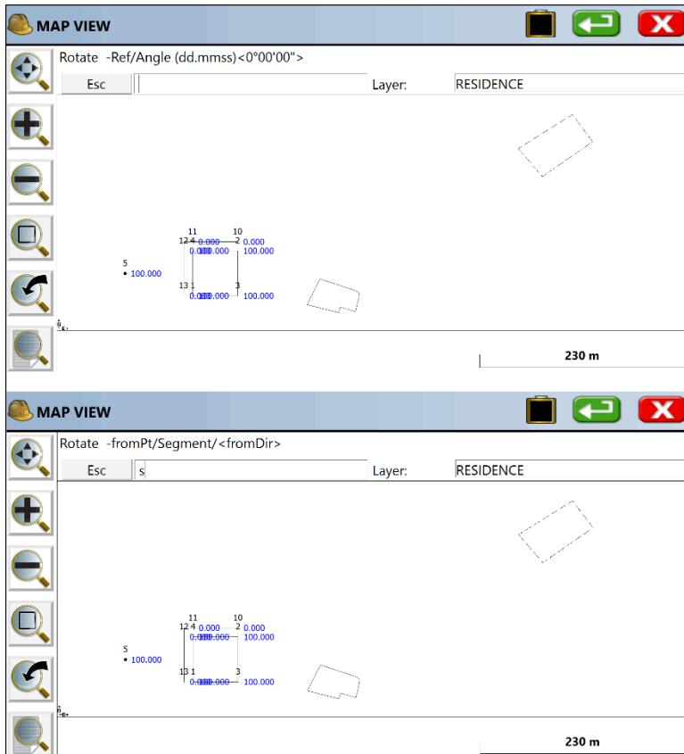
Select the pivot point first. If you want to make it parallel to an existing line, choose R then S for Segment, then pick the segment on the figure you wish to reference first. Then after that, the next pick, also by S for Segment, will be for the property line (e.g. the line to the north) you wish to match.
