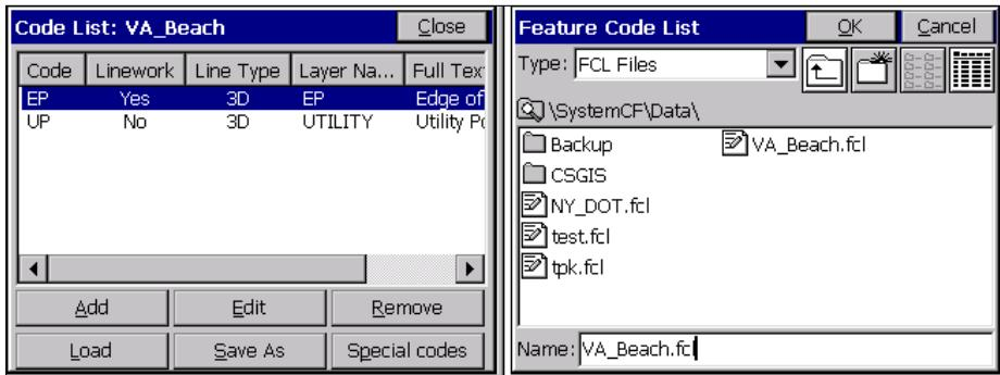
The Add and Edit buttons create or revise Line/Layer drawing properties and GIS prompting. Remove deletes field codes highlighted. Load unloads the current FCL file and loads another existing FCL Field Code List.
