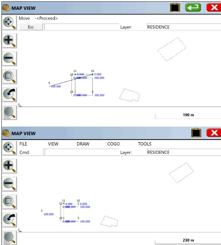
The polylines can be returned to their original position by just reversing the order of the selected Source Point and Target Point. The Copy command may also be used as a Move command, since it has the advantage of showing the new copy and keeping the original, in case you wish to erase the new version and repeat for better results. The Mirror command includes the option to delete the source or retain the source entities.
